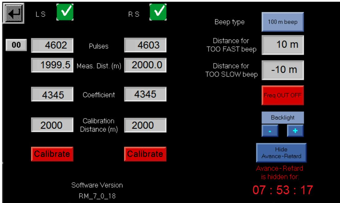
On this page, we can select which sensor(s) to be used for the odometer and to calibrate the instrument for each sensor independently.
