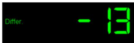
A negative value means that we miss some meters, so we are slow and we have to accelerate, when positive value means we are fast and we have to decelerate. Ideally we have to show continuously 0.
