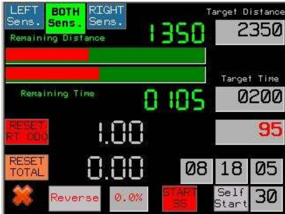
The two bar-graphs give us an idea of our rhythm. In the above example, we see that we are a little bit on delay, as the distance bar is less filled than the time bar.
