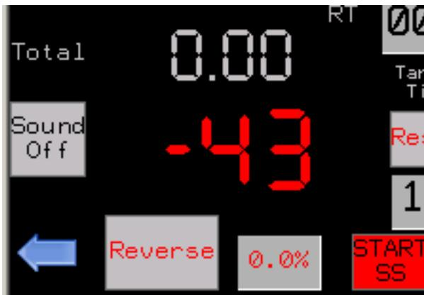
A negative value means that we miss some meters, so we are slow and we have to accelerate, when positive value means we are fast and we have to decelerate. Ideally we have to see continuously 0.
