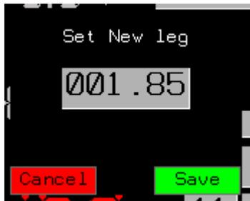
By touching on the grey area a numeric pad appears in order to set the new value to the partial odometer.
