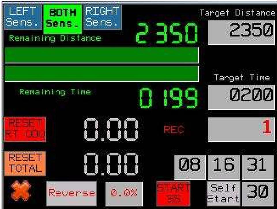
This mode is used in case of rallies of Time-Distance type, with known checkpoints. In the above example, a Target distance of 2.350 m is set and a target time of 200 sec.
