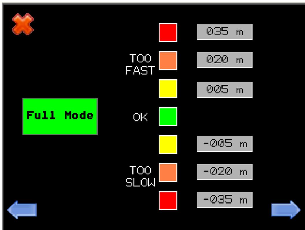
In this page, we can set the distance limits for the Too Fast / Too Slow difference indication. According to this settings, the relative indication will change color on the screen. The lower values (Yellow settings), correspond also to the limits for the sound signal.
