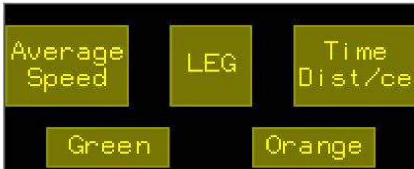
By pressing on the Green or Orange button, the backlight color of the screen can change.
